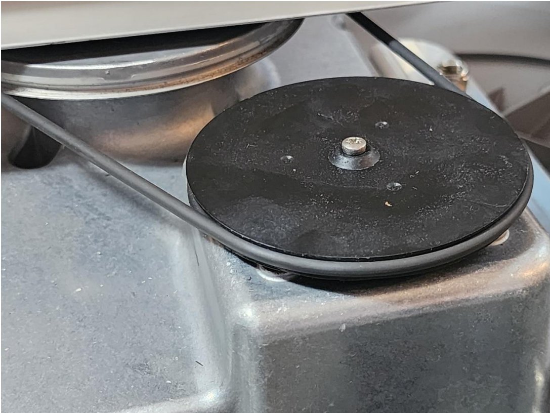
New o-ring drive belt in place.
